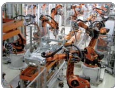
Mig welding robot cell with orbital turntable for welding facia assemblies
