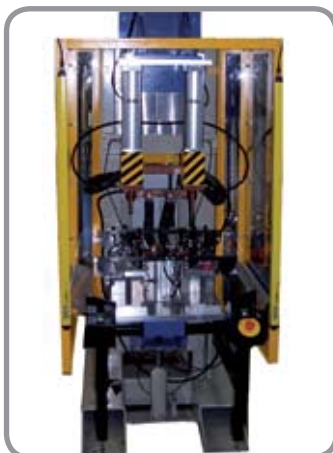
Twin headed projection welding machine with servo controlled fixture for multi component welding
