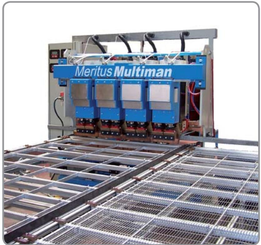
A modular resistance welding system developed for medium to high volume production of flat or profiled panels using pre-cut length wire.
