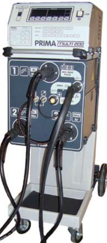
Single sided spot tig tool DRT, with fast earth system DRMT
